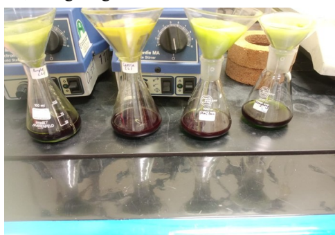
Figure 2. Extracts of Kailan, Purple Kohlrabi Microgreen, Kangkong and Cassia tora being filtered into conical flasks.
