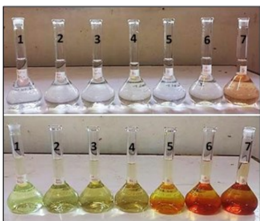
Figure 2. Solutions containing different sample extracts before (top) and after (below) addition of 5% \text{NaVO}_3 . 1 – Blank solution, 2 – Indian mango peel, 3 – Indian mango seeds, 4 – Native guava flesh, 5 – Batuan seeds, 6 – Batuan flesh, 7 – Tamarind flesh
