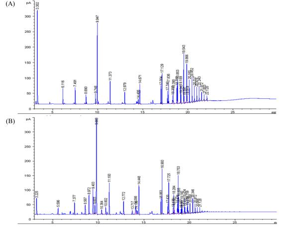
Figure 1. MDAG chromatogram before purification (A) and after purification (B) using the CDT method on a scale of 20 kg
