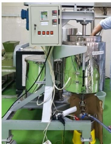
Figure 2. MDAG Purifier scale of 20 kg
