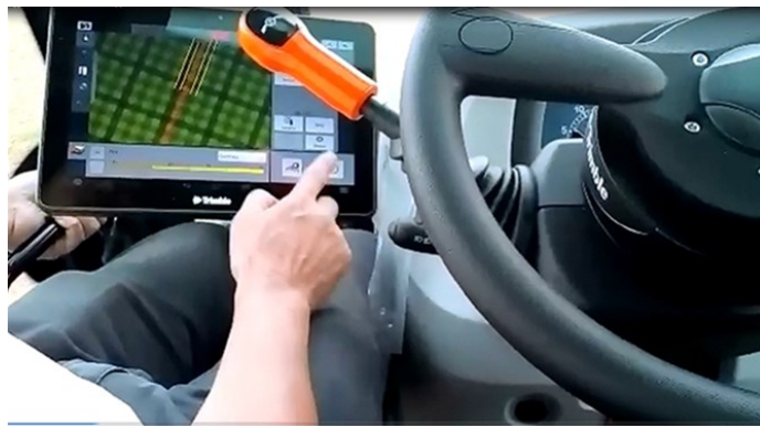
Figure 2. The Trimble® EZ-Pilot® Steering System and Trimble® FmX®2050 Plus Application on the tractor
