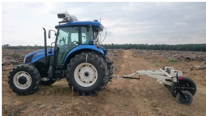
Figure 1. The tractor mounted a Veris 3100 soil electrical conductivity (EC) sensor
