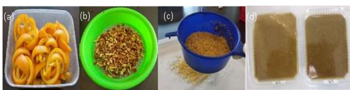
Figure 2. The process of (a) washing and soaking, (b) drying, (c) blend and sieving, and (d) casting for orange peels biofilm production.
