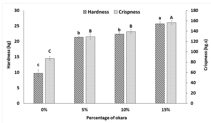
Figure 4. Hardness and crispness of extrudates made with different levels of okara. Bars with different uppercase and lowercase notations represent statistically significant difference ( p < 0.05 ) for crispness and hardness, respectively.
