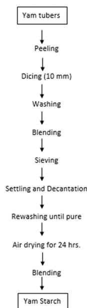
Figure 1. Starch extraction from yam tubers
