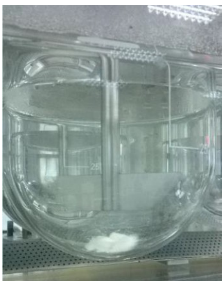
Figure 2. A disintegration test in progress showing the tablet disintegrating into the primary particles.
