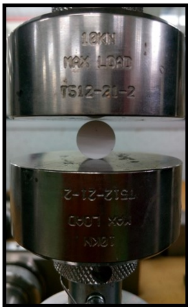
Figure 1. Tablet placed diametrically during the mechanical strength test
