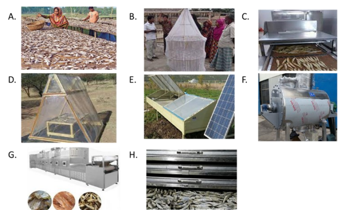
Figure 2. Various fish and seafood drying methods: A. Traditional sun drying, B. Sun drying in ring tunnel, C. Oven drying, D. Solar tent drying, E. Solar tunnel drying, F. Low temperature vacuum drying, G. Microwave vacuum drying and H. Freeze drying
