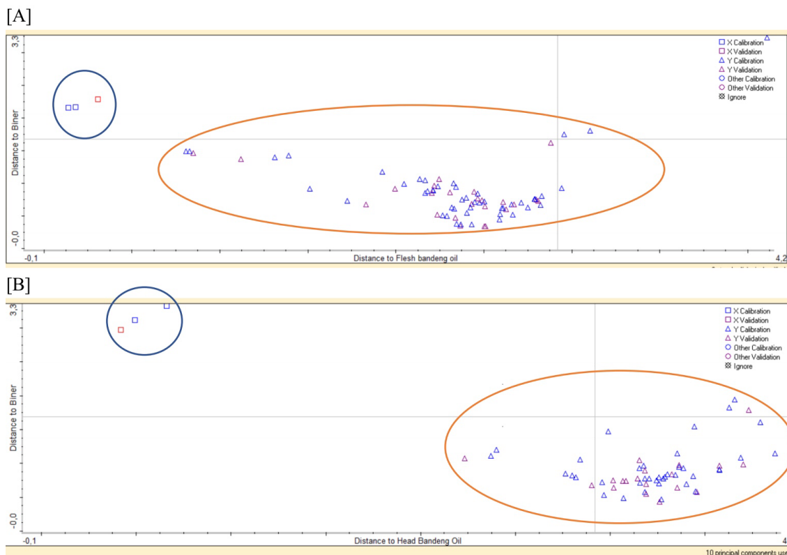
Figure 4. The Cooman plot for discrimination between milkfish fish oil (MFO) [■] and MFO adulterated with palm oil [▲]: [A] Flesh Milkfish Fish oil, [B] Head Milkfish fish oil
