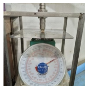
Figure 3. Measuring fracture force using a numerical balance and a system of screw and nut
