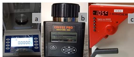
Figure 2. Instruments used for conducting physical properties of coffee cherries and beans (a) Electronic digital balance-SCI-MI-04, (b) Coffee Pro, Moisture-MAC and (c) Electrical oven-binder
