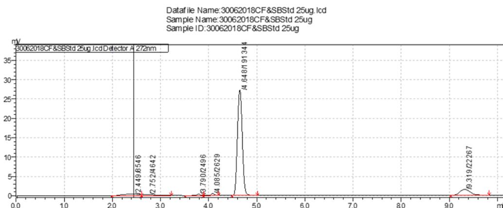
Figure 1. HPLC Chromatogram of 25 µg/L sodium benzoate standard solution
