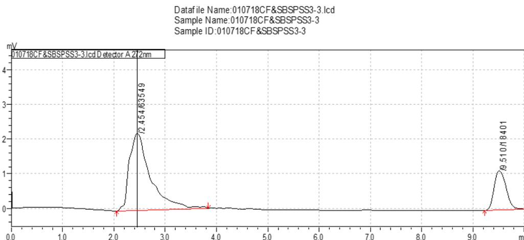
Figure 2. HPLC chromatogram of 20 µg/L sodium benzoate sample solution
