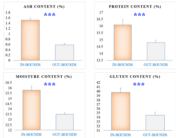
Figure 1. The quality of raw wheat kernels in the tempering bins (in-bounds) and the quality of wheat flour produced after streaming into the flour bins (out-bounds) on Mill A. Values are presented as means of triplicates ( n = 3 ). Error bar shows standard deviation.
