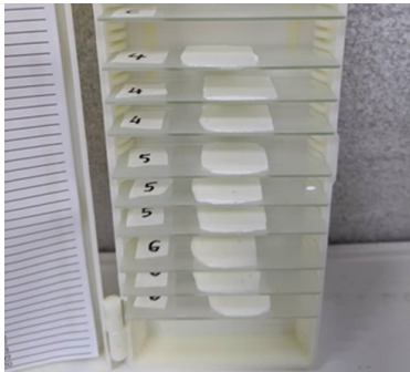
Figure 1. Ice cream samples placed on slides and stored for 24 hrs in -18°C freezer
