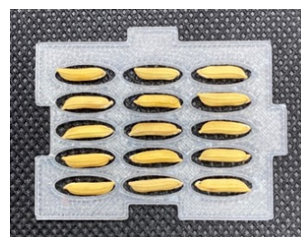
Figure 5. Finalized seed holder with 15 holes per image.
