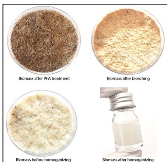
Figure 2. Gradual decolourization through the whole process of PFA treatment, bleaching and homogenization.
