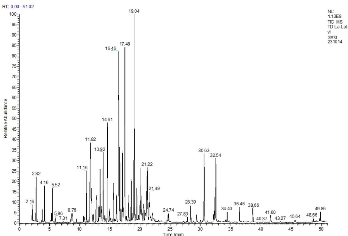
Figure 3. The graph of gas chromatography–mass spectrometry (GC/MS) of lolot pepper essential oils
