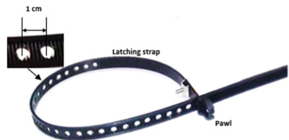
Figure 1. Latching strap. Holes drilled 1 cm apart.
